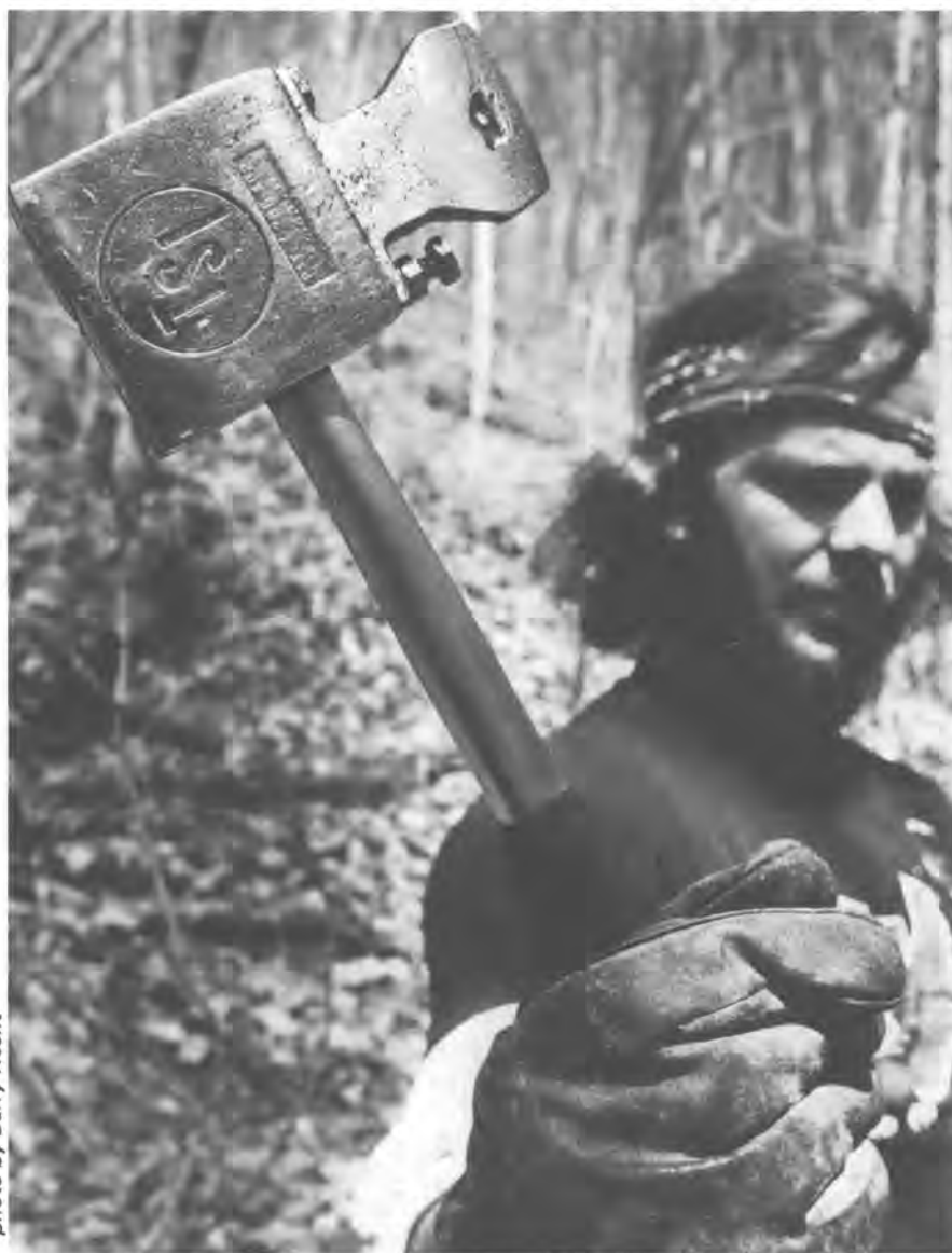
A hypo hatchet is used to inject Tordon into hardwood trees.
